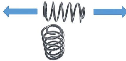
Once you stretch them beyond their **Proof Load** they will not return to normal after removing torque and therefore can no longer apply the proper clamping force when torqued to the same level as previous.
