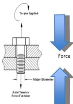
Figure 1. Axial Tension and Clamping Force
